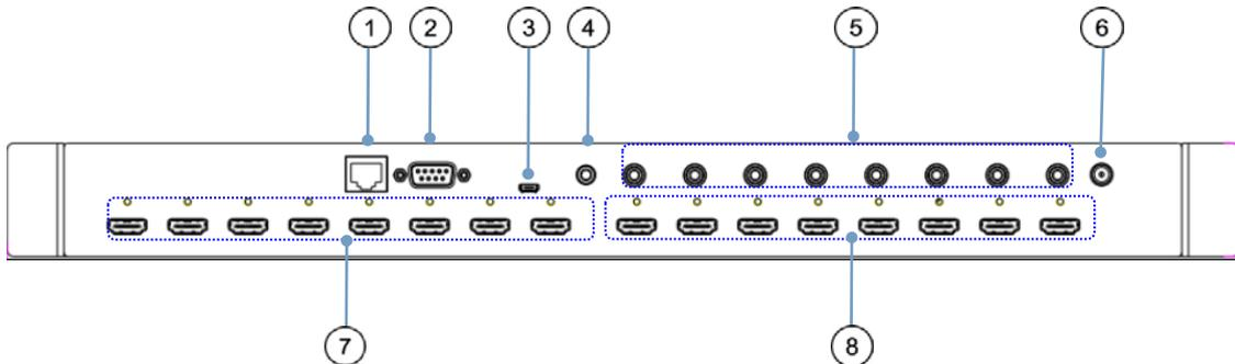
① **IP CONTROL:** Connect directly, or through a network switch, to your PC or laptop to control the unit via telnet/WebGUI.
