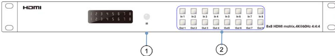
① **IR WINDOW:** Accepts IR signals from the included IR remote for control of this unit only.
