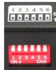
It is a 6 Bit binary switch, when the pin is pull up, its value is "0" ; when pull down, its value is '1". Its default setting is "000000" when you firstly received the units, we mark as group 00 in order to remember easily. Bellow is the group number and DIP setting matching list.
