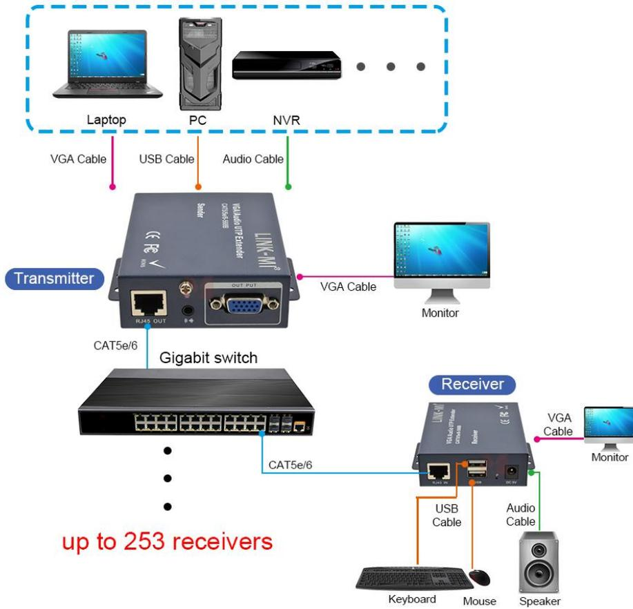
Note: Support transmission modes such as one-to-one/one-to-many. It is not recommended to share the switch with other network devices.
